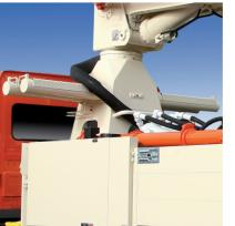
Two slewing cylinders on each side assure safe operation and longevity of the turret.
